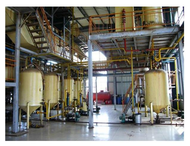
The 5tpd soybean oil refining production line belongs to intermittent refining in terms of refining type, and usually uses chemical refining technology. The processes involved include degumming, deacidification, decolorization and deodorization.
