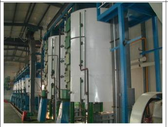
Decolorization tank: Decolorizationtank is usually the tool used in soybean oil refining process to remove impurities such as pigments, metals, and residual soap from the soybean oil. Inhale definite amount of decoloring agent (white clay) into the refined soybean oil, continuously stirring and heating for a period of time.
