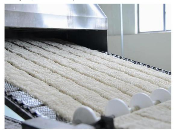
2. Frying time: Frying time is also an important factor affecting the frying effect. It interacts with the oil temperature. If the moisture content in the dough is determined and the oil temperature is low, the frying time will be long; High oil temperature and short frying time. The frying time is too short, the dough is not completely dehydrated, and it is not easy to store; If the time is too long, the dough will bubble and burn, affecting the quality of the dough and increasing costs.
